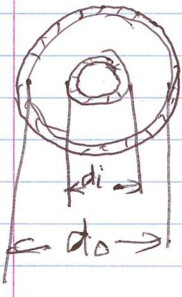
$d_o$  = inside diameter of the outside conductor
